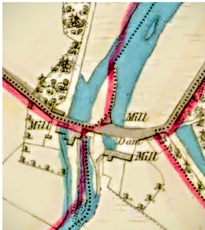
Figure 1. The three mills on the Cregg River, in the townlands of Auclogheen and Drumgriffin, shown on the first edition Ordnance Survey map (c. 1838). Note the several divides in the river, with a stream supplying wheels on each side of the present mill building.
